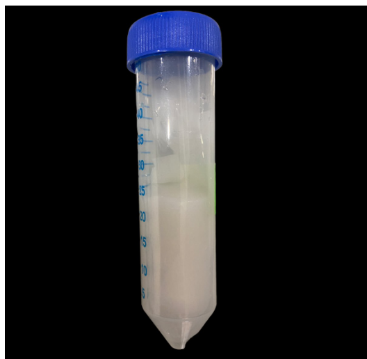
Figure 1. The fabricated hydrogel composed of carrageenan, fucoidan, and titanium oxide nanoparticles
