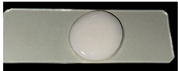
Figure 5. The formulated hydrogel sample was cut and placed onto a clean glass slide for contact angle analysis
