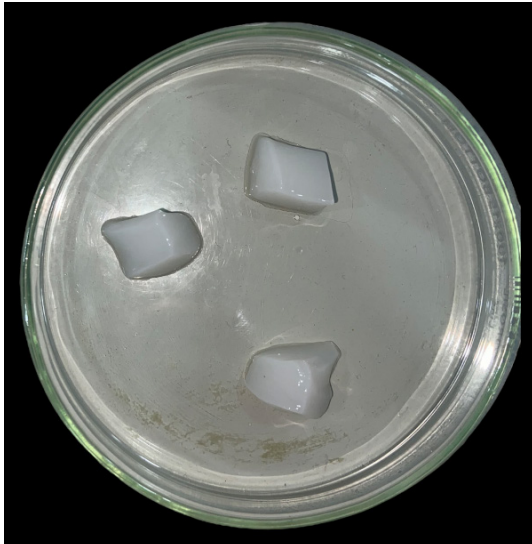
Figure 3. The formulated hydrogel samples are divided into three parts for the subsequent swelling test
