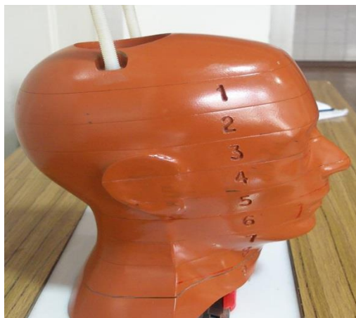
Figure 1. RANDO phantom of the head and neck (Model 706-C; Computerized Imaging Reference Systems Inc., Norfolk, VA)
