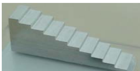
Figure 1. A ten-step aluminum step-wedge
